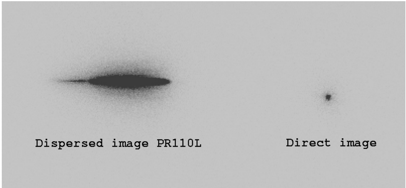
Figure 6.23: Sum of direct (F122M) and PR110L prism exposure of the standard star WD1657+343. The direct image exposure was scaled prior to combination for representation purposes. The cutout shown covers 400 x 185 pixels, where the wavelength increases from left to right for the dispersed image.
