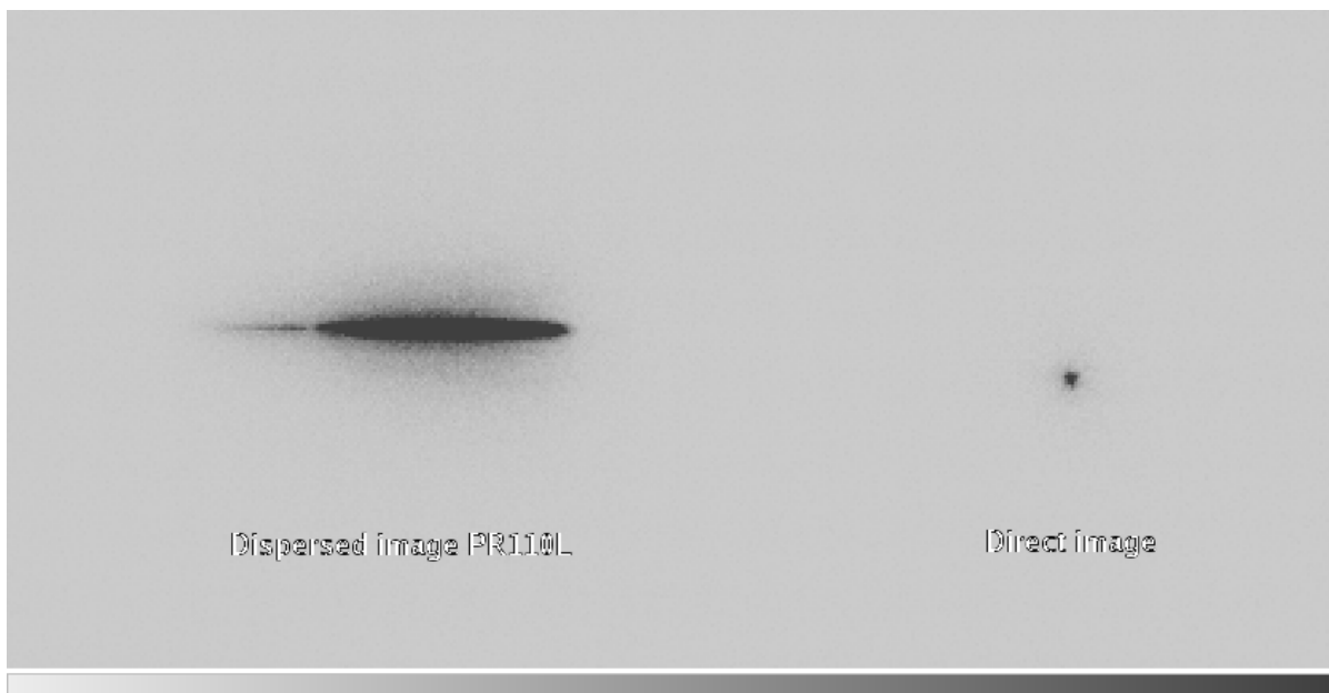
Figure 6.23: Sum of direct (F122M) and PR110L prism exposure of the standard star WD1657+343. The direct image exposure was scaled prior to combination for representation purposes.
