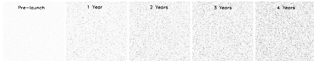
Figure 1.10: A subsection of WFC1 dark frames taken at different epochs showing the increasing population of hot pixels.
