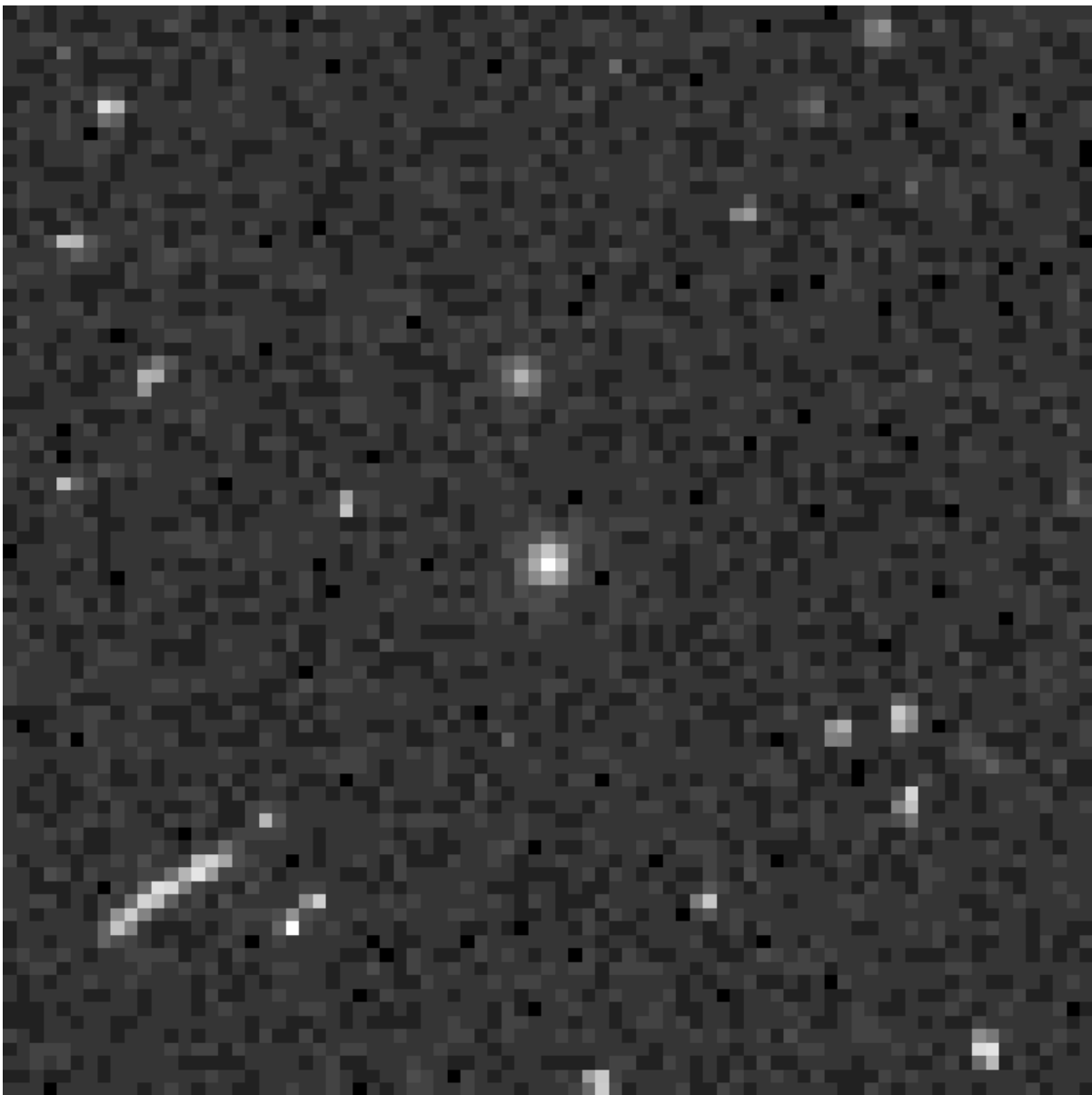
Figure 4.9: Comparison of Star Images and Cosmic Ray Events. An 80x80 pixel subimage of a 400 second F336W WF2 exposure in \omega Cen.
