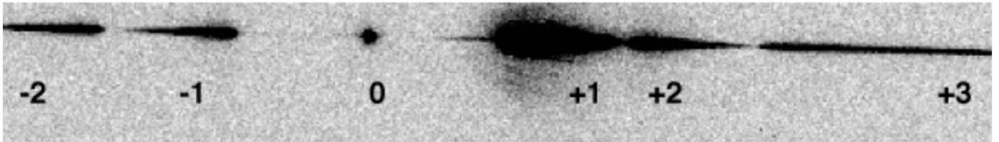
Figure 5.17: Full Dispersed Spectrum for White Dwarf GD153 with WFC/G800L. The numbers indicate the different grism orders.
